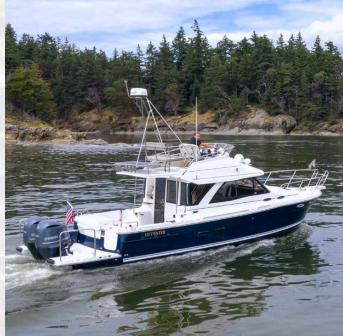
Performance, versatility, and comfort are central to the design of the Cutwater C-32 Command Bridge. The advanced double-stepped, deep-V hull combines speed, efficiency and superior stability. Our Laminar Flow Interrupters allow for smooth, positive cornering. Roll the throttles forward and you'll feel the powerful twin, counter-rotating 300 HP Yamaha outboards propel the C-32 CB to remarkable speeds. Docking is easier than ever with Helm Master joystick steering.
